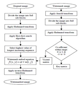
Fig.4 Flow Diagram for Watermark Embedding Process
