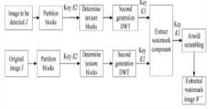
Fig 3. Digital watermark extracting algorithm flowchart
