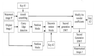
Fig 2. Digital watermark embedding algorithm flowchart
