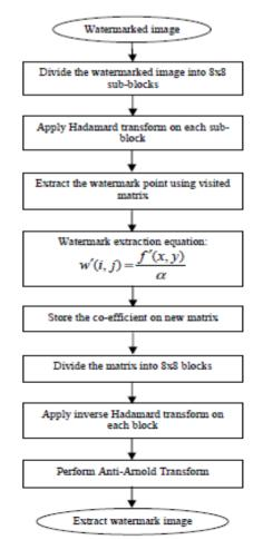
Fig.5 Flow Diagram of Watermark Extraction Process
